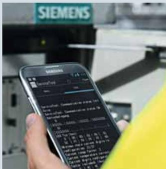
After the connection has been established, all ServiceTool functions are available in parallel on the technician's smartphone on site and on the screen in the Service Center.
